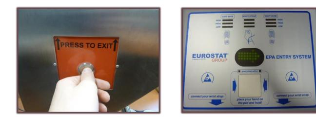
To quit the EPA, no test is needed. Push the button on the side of the turnstile, the top screen displays a green arrow which indicates the exit direction.
