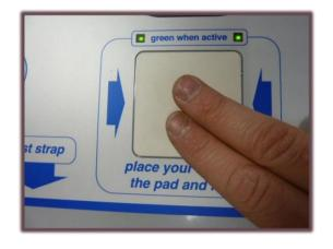
The measurement starts by touching the sensitive electrode on the top of the turnstile. A "bip" sound and two green LEDs indicate the beginning of the test
