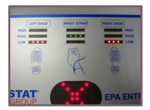
When the measurement is finished, three LEDs display show the resistance value of each equipment.
