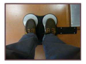
Step on the footplate for testing the ESD shoes.
